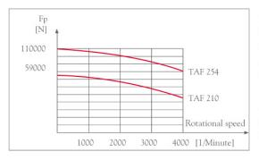
At increasing rotational speed there is an existing danger that the clamping force may decrease, due to this the workpiece may slip in the chuck, maybe even fly out. The clamping force is depending in a high measure on the lubrication status, on the quality of the lubricating grease, on the height of chuck jaws and on other factors.
