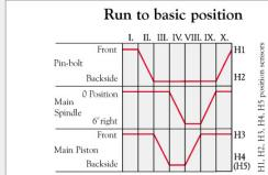
The diagrams demonstrate well that the adjustment of the chuck jaws are performed by the cyclical, well-adjusted actuation of the three elements (the pin-bolt switch elements, the turning of the lathe machine main spindle by 10° from the "0" position, and the move of the hydraulic cylinder that is actuating the chuck), realising by this the principle of function-pooling as well.
